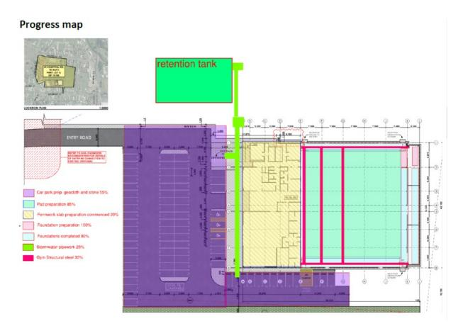
3.8 The carpark sub-base construction is well advanced with placement and shaping of basecourse to finish levels underway. Installation of steel framing to the gymnasium area is well underway and formwork to perimeter of amenities area is progressing.
